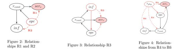
Given  $(opc, r_{cont}) \in R$ , any operational fault caused by an error provoked by an entity may sooner or later trigger a disruption on  $ser_c$ . This is due to the transitive dependency relationship described below (R1) and which is also depicted in Figure 2.
