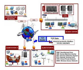
Figure 1: A Current SCADA Network Architecture
