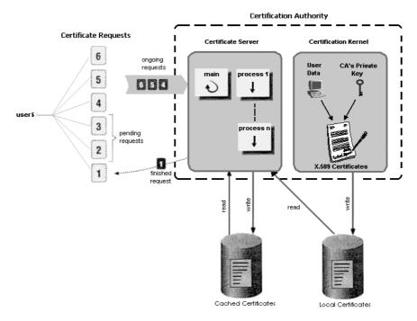
Figure 1. Composition of a Keys Service Unit
