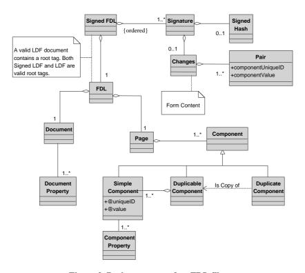
Figure 2. Basic structure of an FDL file
