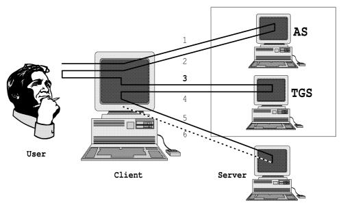
Figure 1 The Kerberos authentication protocol.
