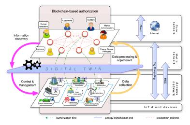
Figure 2: B5G-enabled Smart Grid architecture for accommodating DTs in the long term
