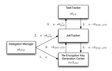
Fig. 2. Re-Encryption Key Generation protocol
