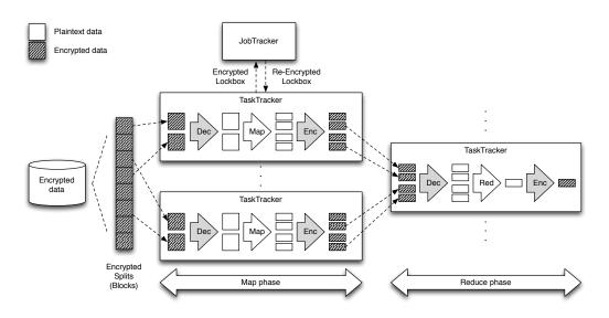
Fig. 3. Operation of our proposal during the consumption phase
