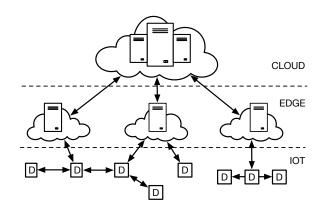
Fig. 1. Edge Computing Architecture
